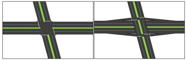
Figure 1: Current intersection (left) and upgraded grade separated intersection (right)
